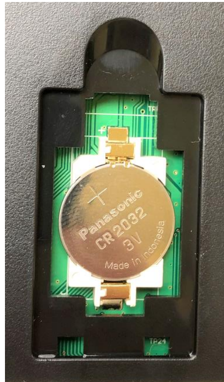
Step 3: Battery installation
