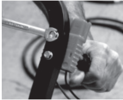
Secure charging Quick Connect to upper handle.
